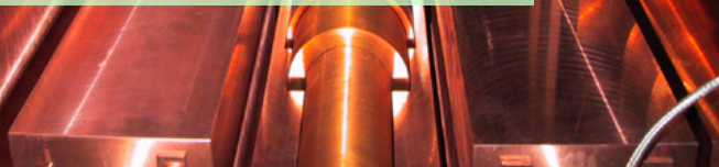
detectors during installation; in the central and right up detectors the new shaped Cu shield surrounding light guides (acting also as optical windows) and PMTs was not yet applied
