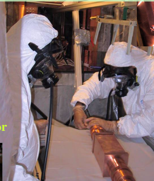
installing DAMA/LIBRA detectors
