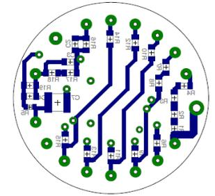
Design of the voltage divider and preamplifier mounted on the Pyralux support
