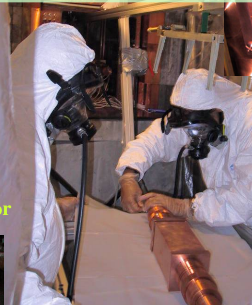
installing DAMA/LIBRA detectors
