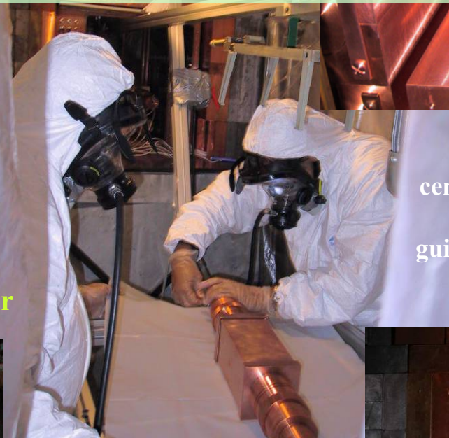
installing DAMA/LIBRA detectors
